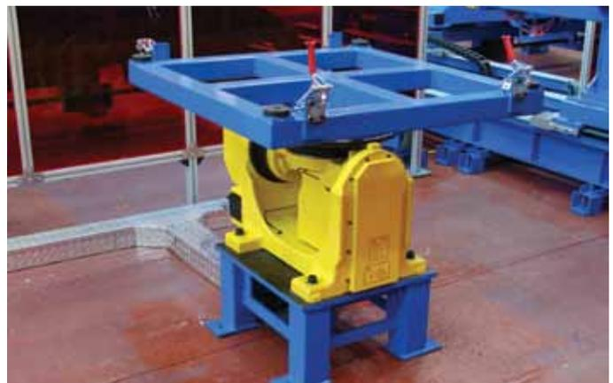
A two-axis manipulator installed in order to improve access to some of the more complex components and to achieve as much flexibility as possible.
