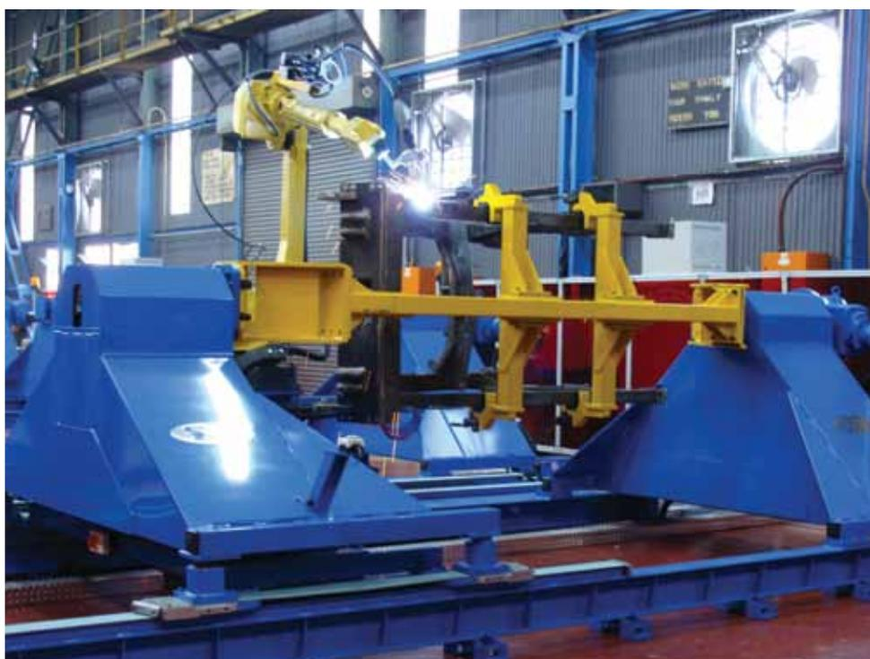
A wheel module component being welded at the front-end workstation.
