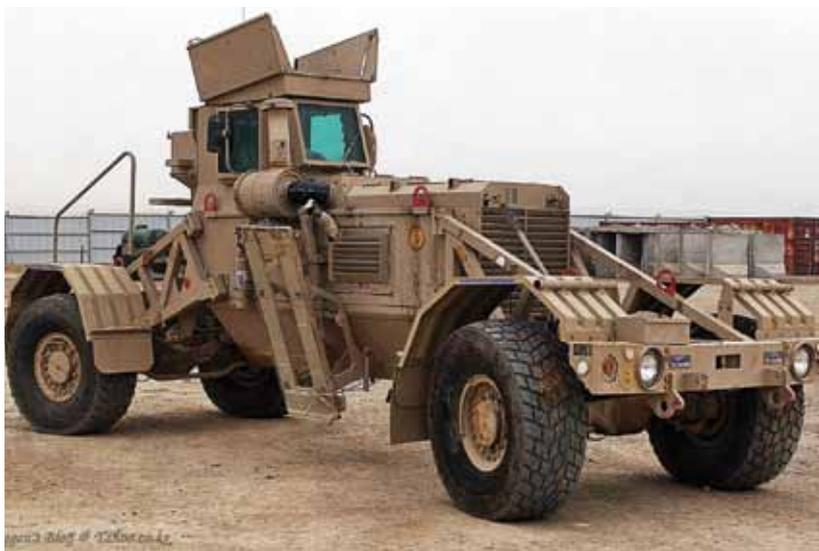
The South African-designed and manufactured mine detection vehicle that can detect mines while travelling at 25 km/h. (Image from: [img.blog.yahoo.co.kr/ybi/1/24/56/shinecommerc](http://img.blog.yahoo.co.kr/ybi/1/24/56/shinecommerc)).
