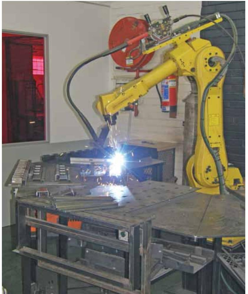
The Fanuc Roboweld 120 iB coupled to a Lincoln 455 power source making parts at AlClad’s Steeldale facility in Johannesburg. Traditional jigs are made and used to weld parts on five worktables in front of the robot.
