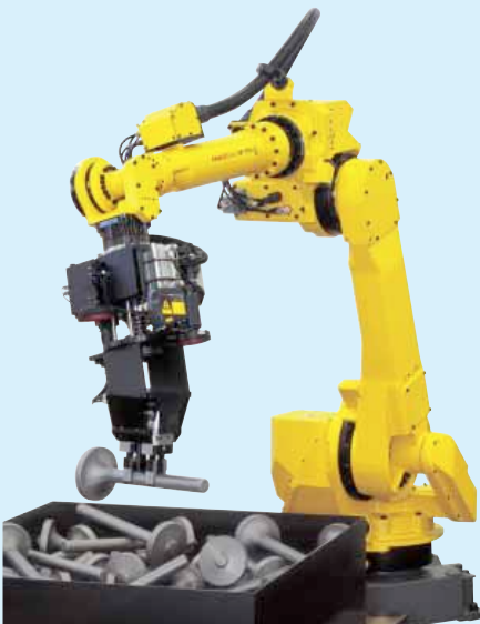
Bin picking of cylindrical parts by M-710iC/50
