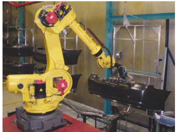
A first-of-a-kind robotic system to transfer bumper parts from the washing bay system onto the paint system. Venture in Wadeville, South Africa is the only manufacturer in the world that does not depend on humans for this application.
