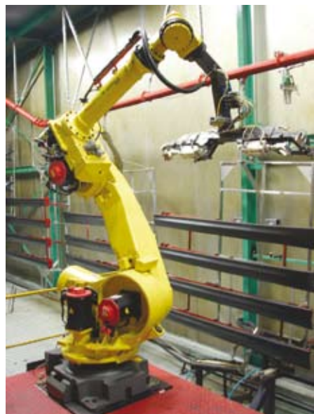
The pick-and-place robot system with its unique gripper – shown transferring injection moulded side-skirts for BMWs.
